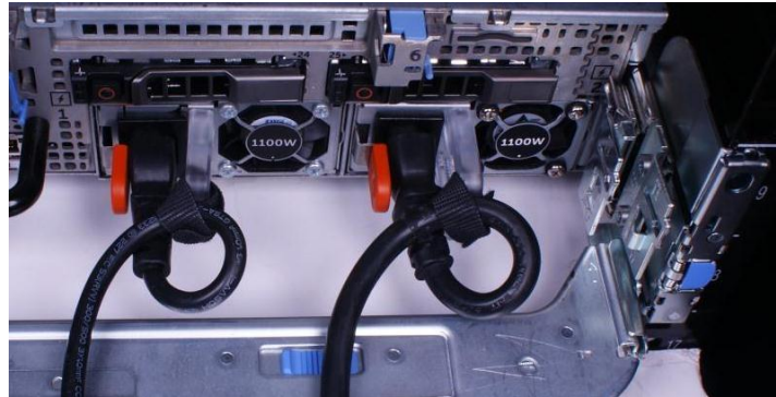
Figure 2. Routing power cables through the strain reliefs
